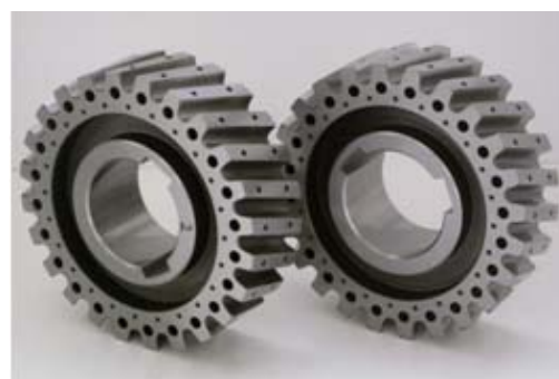
Fig.5 Photograph of tested gear wheels designed for centrifugal lubrication
