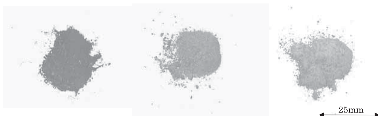
Fig.4 Appearance of the Bizen Soil E. Left: before HT (raw soil); Center: after HT at 1000^\circ\text{C} ; Right: after HT at 1260^\circ\text{C} (faragmented Bizen Yaki). HT means "Heat Treatment".
