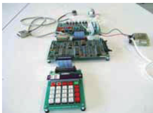
Fig.2 Experiment equipment of Z80 microcomputer
